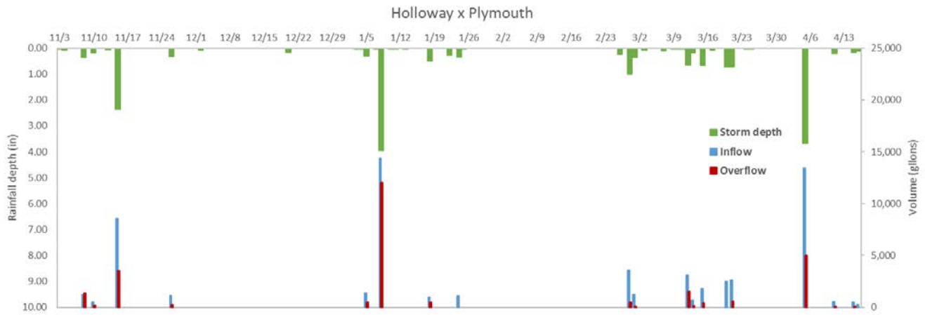
Figure 9: Hydrograph showing inflow and GI overflow of the 2017-2018 Monitoring Period at Holloway x Plymouth
