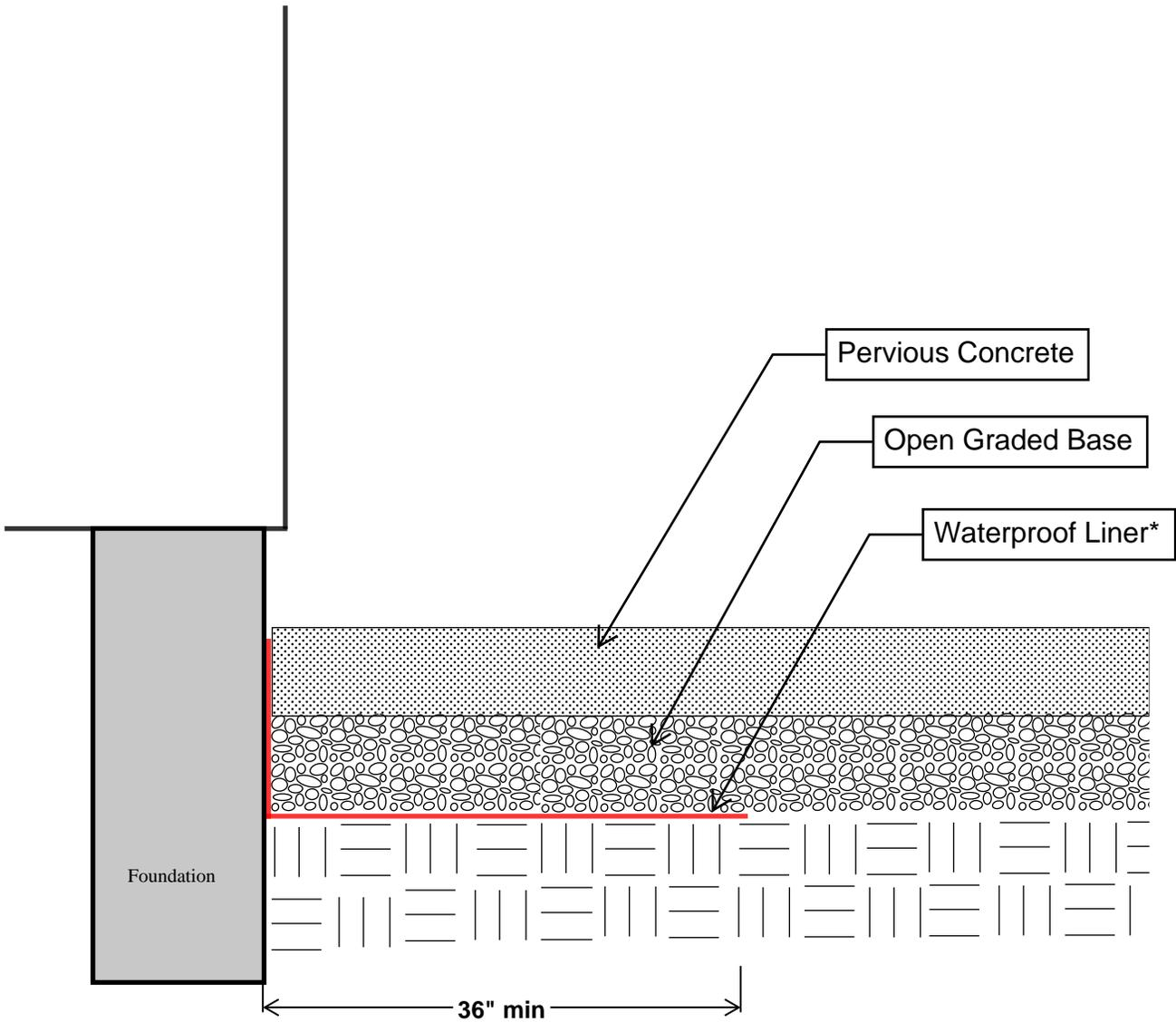
\* Ground contact rated membrane, i.e.: Permilon PLY-X-150 / Moistop Ultra-15
